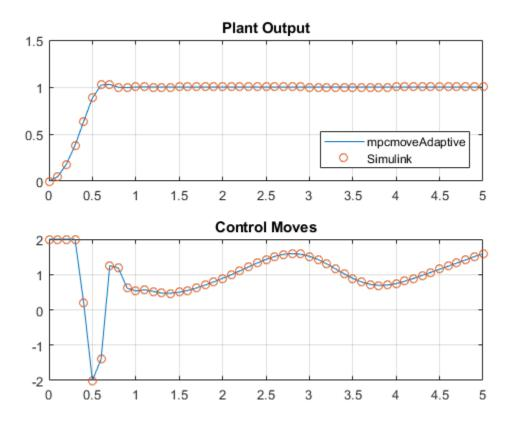
The closed-loop responses in MATLAB and Simulink are identical.
