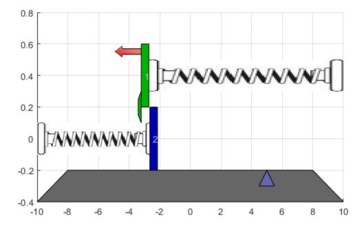
When the masses are not connected, MPC2 applies excessive force since it expects a larger mass. This aggressive control action produces oscillatory behavior. Once the masses connect, the control performance improves, since the controller is designed for this condition.
