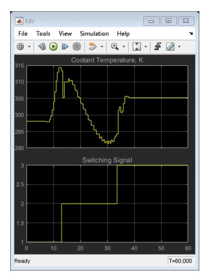
The transition is now well controlled. The major improvement is in the transition through the open-loop unstable region. The plot of the switching signal shows when controller transitions occur. The MV character changes at these times because of the change in dynamic characteristics introduced by the new prediction model.
