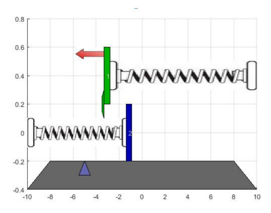
Both masses move freely until they collide. The collision is inelastic, and the masses stick together until a change in the applied force separates them. Therefore, there are two operating conditions for the system with different dynamics.
