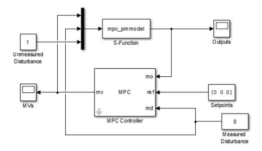
The MPC Controller block controls the nonlinear paper machine plant model, which is defined using the S-Function  $\tt mpc\_pmmodel.$
