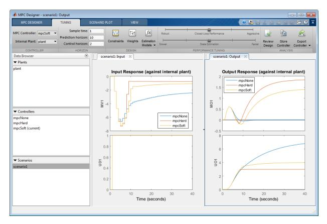
The response plots update to reflect the new mpcSoft configuration. In the **Output Response** plot, mpcSoft shows a compromise between the previous controller responses.
