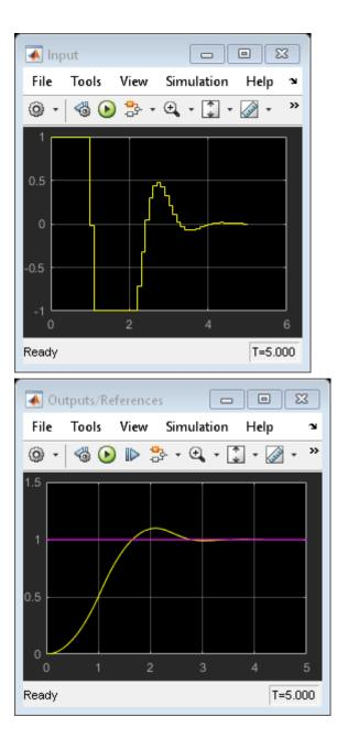
Simulate with Explicit MPC controller in Simulink. Controller "mpcobjExplicitSimplified" is specified in the block dialog.
