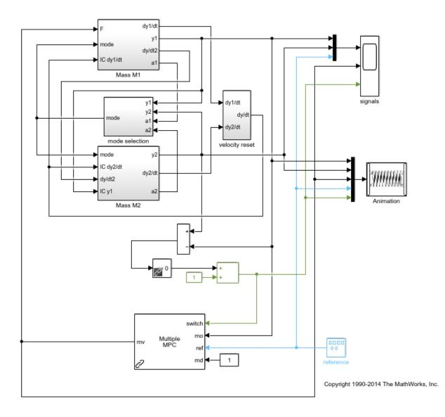
In the model, the Mass M1 subsystem simulates the motion of mass M1, both when moving freely and when connected to M2. The Mass M2 subsystem simulates the motion of mass M2 when it is moving freely. The mode selection and velocity reset subsystems coordinate the collision and separation of the masses.
