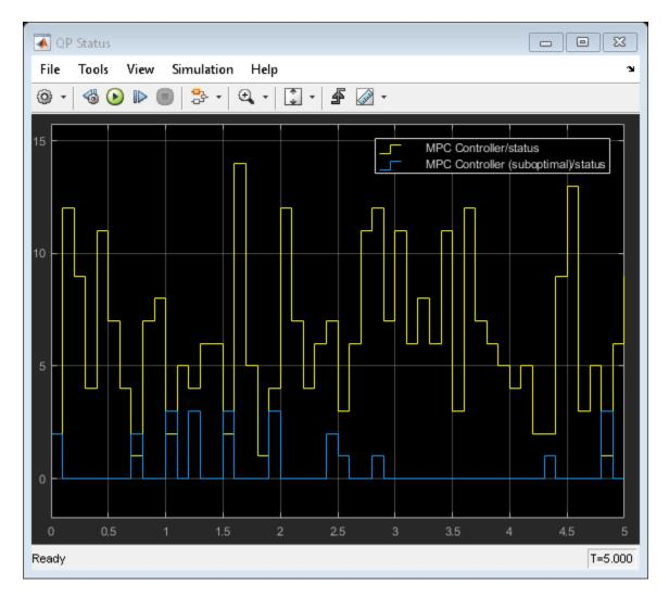
As in the command-line simulation, the average number of QP iterations per control interval decreased without significantly affecting control performance.
