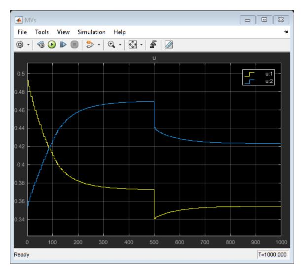
In this example, you are able to calculate the steady-state  $u_1$  and  $u_2$  that maximize the C2H4O production rate ( $y_1y_2$ ) for a given C2H4 availability ( $u_4$ ) and reactor temperature ( $u_3$ ).
