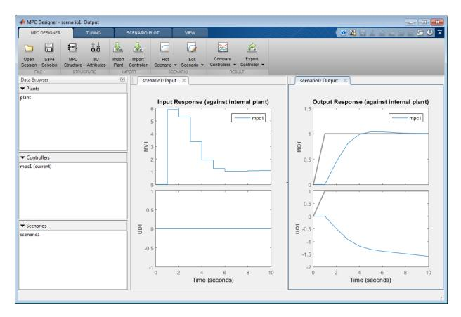
The app adds the specified plant to the **Data Browser** along with a default controller, mpc1, and a default simulation scenario, scenario1.
