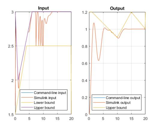
The results of the command-line and Simulink simulations are the same. The MPC controller keeps the input and output signals within the specified bounds as the constraints change throughout the simulation.
