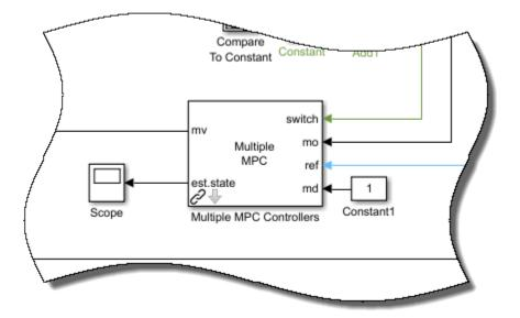
Define the state ranges for the explicit MPC controllers based on the ranges of the estimated states.
