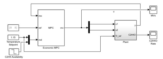
C2H4 availability is initially 0.175 and remains constant for the first 500 seconds, which allows the controller to drive the plant to a new steady state with higher C2H4O production. C2H4 availability then steps down to 0.15 at t = 500 and remains constant for another 500 seconds. The economic MPC controller again maximizes C2H4O production at this condition.
