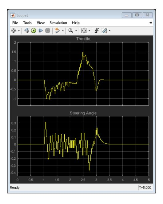
The simulation result is identical to the command-line result. To support a rapid prototyping workflow, you can generate C/C++ code for the blocks in the obstacle avoidance system.
