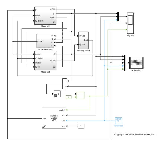
To specify the explicit MPC controllers, double-click the Multiple Explicit MPC Controllers block. In the Block Parameters dialog box, specify the controllers as a cell array of controller names. Set the initial states for each controller to their respective nominal value by specifying the states as { '[], '[]'}.
